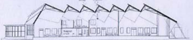
Fig.6 Section showing change in solar access due to the specially designed roof opening
